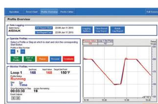
SpecView is designed for industrial users with features such as data logging, trending and support for bar code readers and touch screens. Errors are reduced, for any process, by creating application-specific screens. The software provides a historical replay option, easy-to-use recipe features and remote access options, including LAN, Internet and modem.
