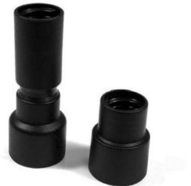
Static conductive hose connectors are impregnated with carbon black to make them conductive. These connectors are used to connect two bare hose ends. They have a female thread to accept vacuum hose on each side.
